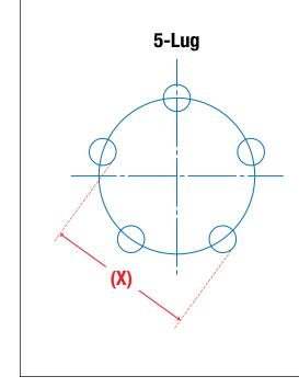
Measure from the inside of one hole to the outside of the farthest hole. Use the chart below to find your Lug Pattern/PCD.
